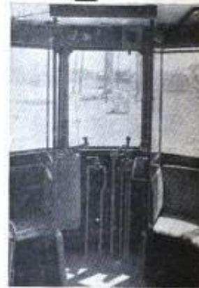
The Master Controller and Control Switch in Cab. All other Circuit-Breaking Devices are beneath the floor.
